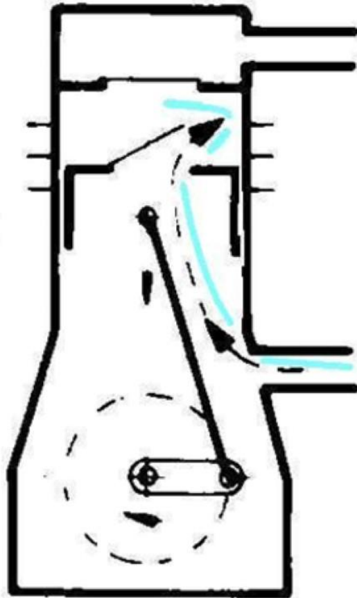
Unidirection compressor. Suction from the crankcase
